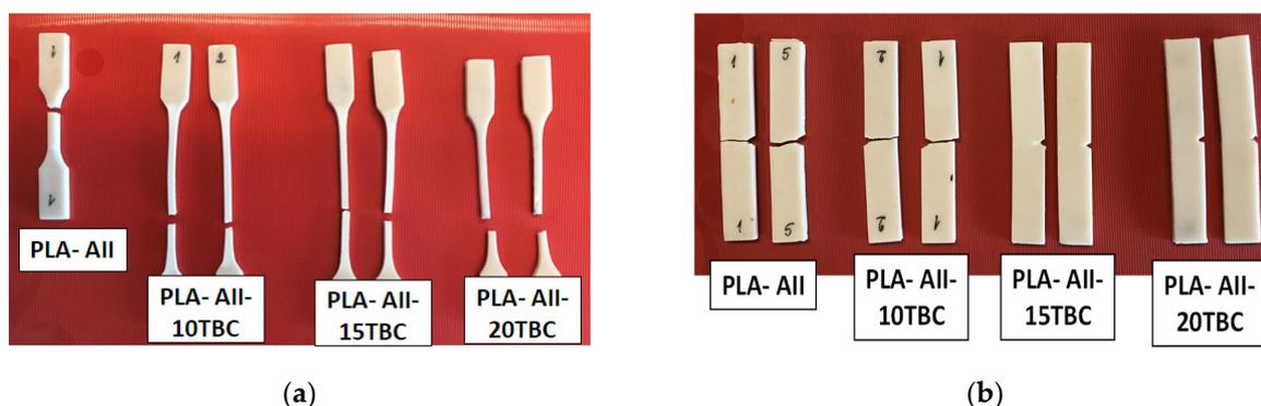
**Figure 10.** (a,b) Pictures of PLA/AII specimens (with/without plasticizer) to illustrate their aspect after the mechanical characterizations: (a) tensile and (b) Izod impact testing.
